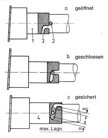
After connecting the quick lock couplings make a visual check that the collar is extended forward over the bearing far enough for the safety pin to engage.
